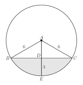
Since  $\cos(\angle DAC) = \frac{3}{6} = \frac{1}{2}$ , we see that  $\angle DAC = 60^{\circ}$ . Therefore,  $\angle BAC = 120^{\circ}$ . The
